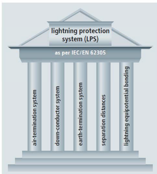
Figure 4.1 Components of a lightning protection system
